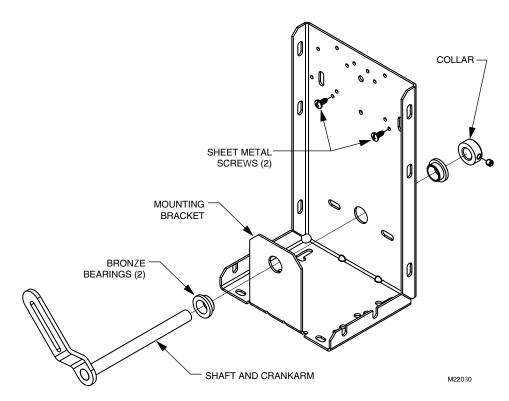
Fig. 3. Mounting kit exploded view.
