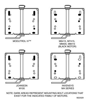
Fig. 2. Foot-mount hole usage.
